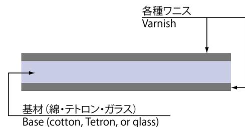
FIBREX is constructed from a base on which the varnish is coated and dried. All materials are of the non-adhesive type and it is possible to slit and cut the original material into necessary table sizes.
